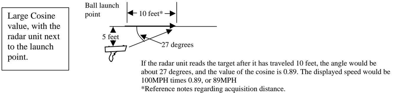
To reduce this, move behind the launch point and keep the radar unit in the line of ball travel.
