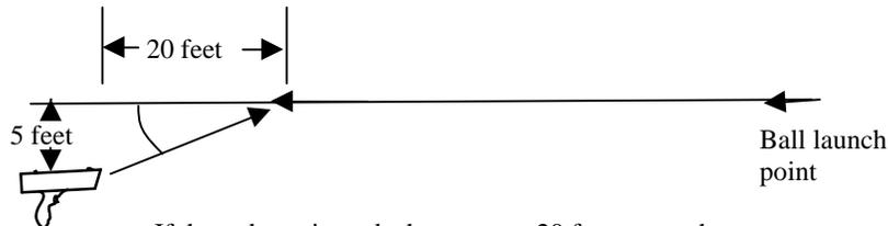
If the radar unit reads the target at 20 feet away, the angle would be about 14 degrees, and the value of the cosine is 0.9703. The displayed speed would be 100MPH times 0.9703, or 97MPH
