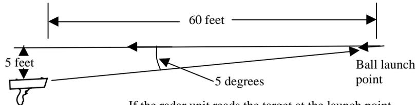
If the radar unit reads the target at the launch point, the angle would be about 5 degrees, and the value of the cosine is 0.9965. The displayed speed would be 100MPH times 0.9965, or 99.7MPH (which would round up to 100MPH).
